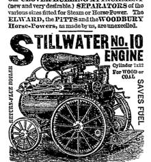
MINNESOTA GLANT FARM ENGINES. each having return-flue, and fitted for burning straw, wood or coal. These Engines are made and finished in the most perfect manner. TRACTION ATTACHMENTS can be furnished with any of
