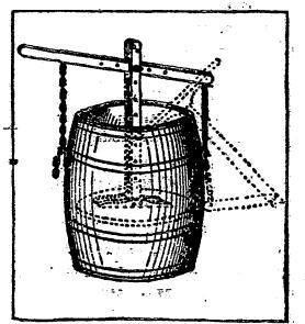
brine when removed can be placed in position to drain into the barrel, the dotted lines in the illustration showing the position when the press is re-
