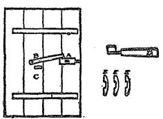
THE LATCH IN PLACE. ed one is shown in the cut. The picture shows the inside of the door. A is the latch, B the piece that drops down and unlocks it when it is punched forward by means of a pin which fits in the latch in the ordinary way; D is the key and C the keyhole. EEE are the wooden pieces in which the latch works. This latch could be made with a very few tools and will de the work.
