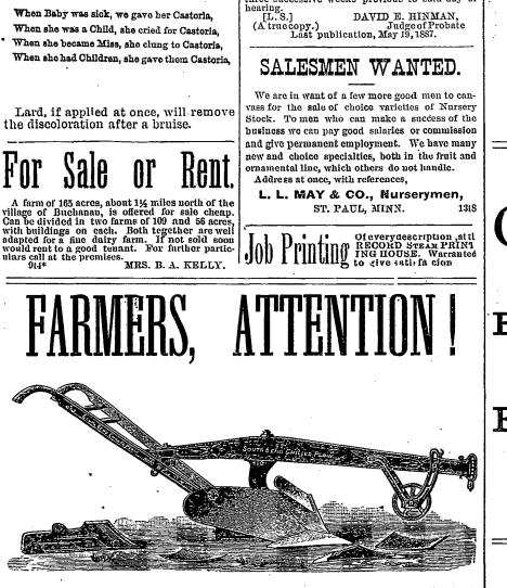
This is a fair representation of the South Bend Chilled Plow Company's new Plow, with the latest improvements in Reversible Point, Patent Jointer, and Drop Land Side, not used in any other plow. Call and see it.
